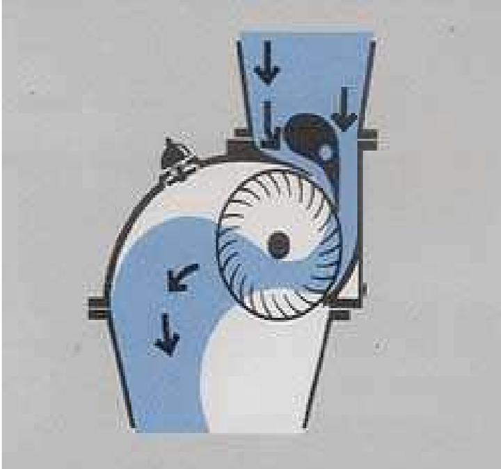
A crossflow turbine is an impulse turbine, relying on the kinetic energy of the water striking the blades to spin the turbine.
